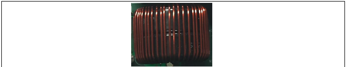
Figure 4 Main PFC inductor
